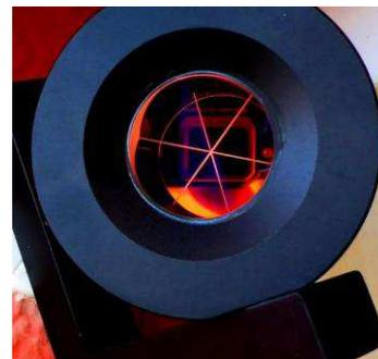
Monitoringprisma - Leica Geosystems
